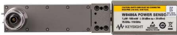
Figure 4. W8486A comes without built-in EEPROM. Users need to pre-enter calibration factors printed on the back of the sensor into the power meter.
